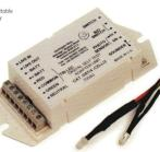
Dimensions Height: 30mm x Length 130mm x Width 50mm, Fixing centres: 120mm, Weight: 80 grams.
